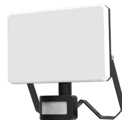
Smart Frameless Security Light Tunable White Art. # 54 01 0008 00 EAN 8712879149750 20W, 3000-6500K, 2500 Lumen, IP54 Sensor Range: 10m / Sensor Angle: 120°
