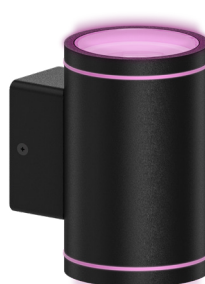
Smart LED Up & Down Light RGB+Tunable White Art. # 54 01 0005 00 EAN 8712879149569 2x4W, 2x380 Lumen IP54
